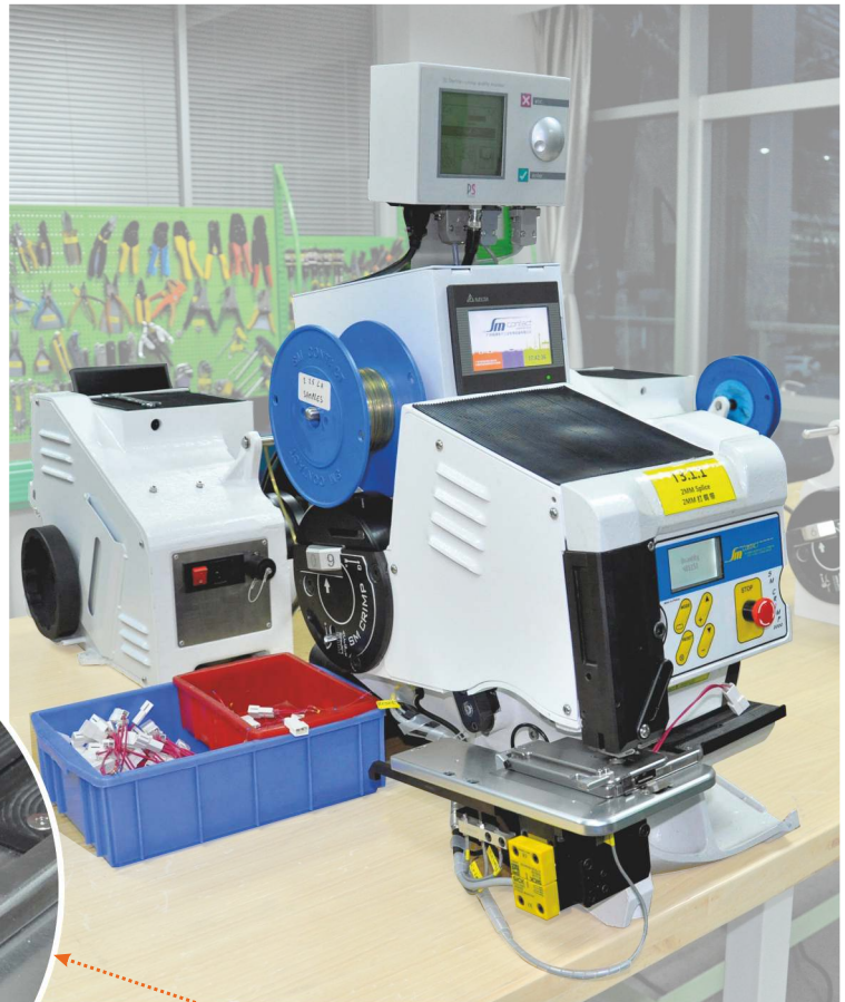
Automatic table with exchangeable jig for splice crimping of 2 sensors with wires
